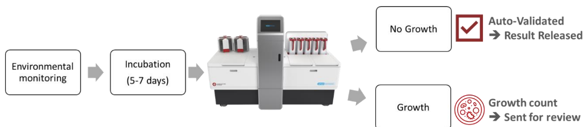
Figure 1. High level workflow of the APAS in a QC laboratory
